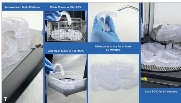
Fig. 7: Following the right protocols according to the manufacturer's instructions is key. IPA = isopropyl alcohol.
