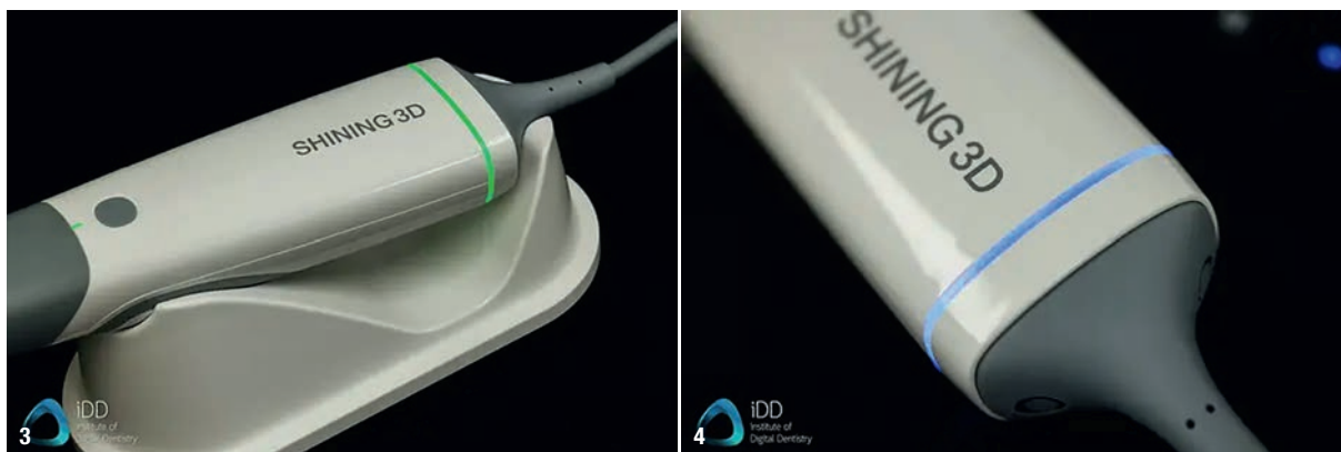
Figs. 3 & 4: The LED ring shows the scanning and connection status.
