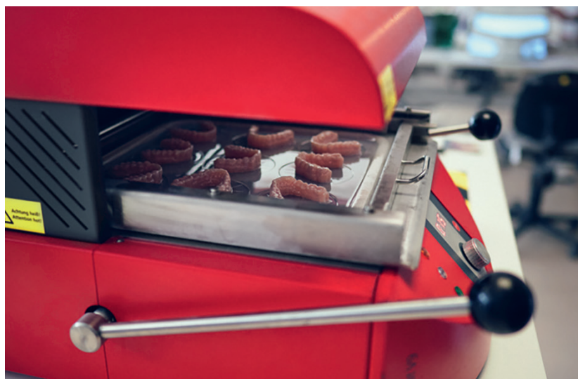
The tooth models that serve as the basis for manufacturing each step of the aligner treatment are 3D-printed. (All images: © PlusDental)
