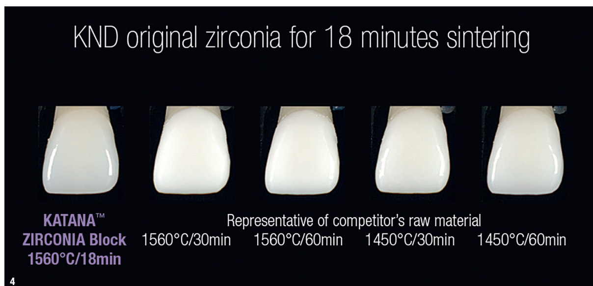
Fig.4: The KATANA Zirconia block displays superior optical properties after 18 minutes of sintering compared with representatives of major competitors' raw material after 30-minute and 60-minute sintering programmes designed by Kuraray Noritake Dental based on the manufacturer's recommendations.
