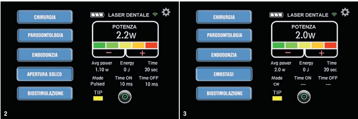
Fig. 2: The settings of the 980nm diode laser used with single-use fibres. Fig. 3: The laser settings for completely drying the sulcus with a programme in continuous-wave mode.
