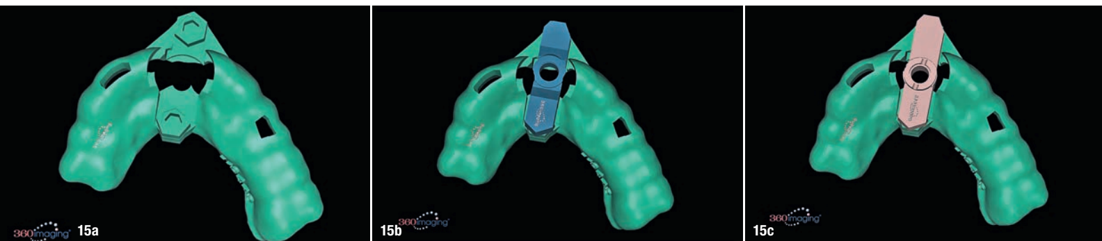
Fig. 15a: The base template was designed to seat firmly on the adjacent teeth, incorporating buccal and lingual hexagonal offsets to engage the different drill guide inserts. Figs. 15b & c: Separate inserts were fabricated for the initial drill guide to reach the root apex to accommodate sectioning, followed by a second guide for final osteotomy drilling and implant placement.
