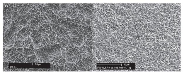
Fig. 2a: The SLA® surface of Straumann® titanium implants. Fig. 2b: The ZLA® surface of the Straumann® PURE Ceramic Implant System.
