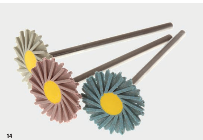
Figs. 14 & 15: Silicone brushes with diamond grains do not change the shape of the surface, but smooth it. Contact with the workpiece should be made at a slight angle so that the bristles can deflect better and do not kink.
