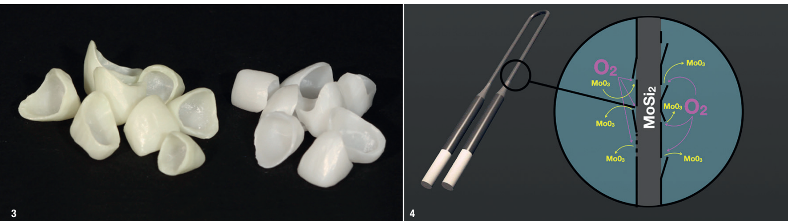
Fig. 3: Restorations displaying greenish surface pigmentation. Fig. 4: A molybdenum disilicide heating element with a protective silica layer bursting off, leading to pest oxidation and contamination of the elements in the sintering chamber. MoSi 2 = molybdenum disilicide; O 2 = oxygen; MoO 3 = molybdenum oxide.
