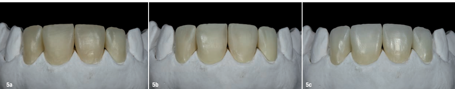
Figs. 5a–c: Effect of temperature differences during sintering on restorations made of KATANA Zirconia UTML: the restorations were sintered at the same nominal temperatures in three different furnaces.
