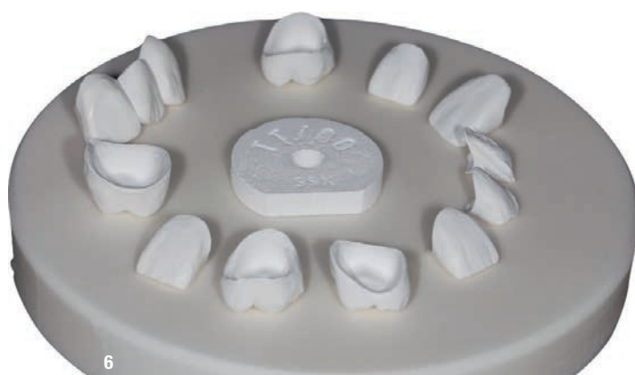
Fig. 6: TempTAB on a sintering tray with restorations ready for sintering.
