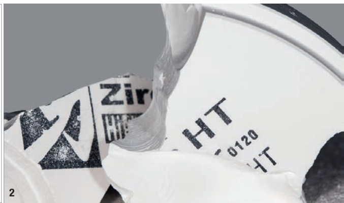
Fig. 1: Alumina sintering beads may be the cause of white spots on a restoration surface if not replaced on a regular basis. Fig. 2: Pieces of a white zirconia blank left over after milling.
